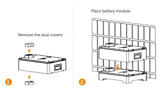
\*Note: If the Base is shifted after placing battery module, move it to its original location according to the mark previously drawn.
