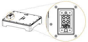
The hot-plug interface is connected to the bottom of battery module.
