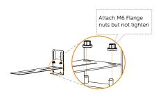
Step 7. Secure the assembled bracket on the battery module and wall.
