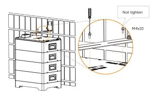
Move the assembled bracket to the wall;
