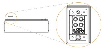
The hot-plug interface is connected to the bottom of battery module or BMS.
