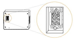
The hot-plug interface is connected to the top of battery module or Base.
