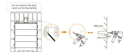
Remove the assembled bracket; Insert Expansion bolt (Part N) (x 2 pcs)
